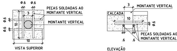
DETALHES DA ANCORAGEM DOS MONTANTES VERTICAIS NA CALÇADA ESCALA 1:5 MEDIDAS EM CENTÍMETROS
